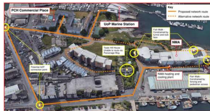
Figure 29: Sutton Harbour pipework routing options and constraints
