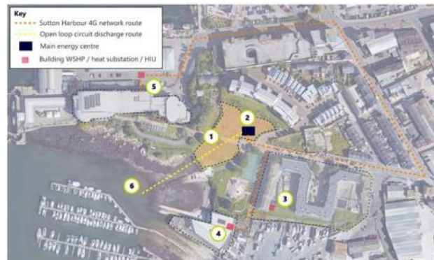
Figure 38: Location plan for scenario 3a - Open loop ground source 4G network and connections
