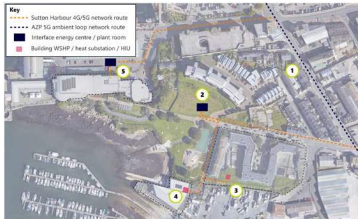
Figure 1: Location plan for scenario 2 - AZP 4G network and connections
