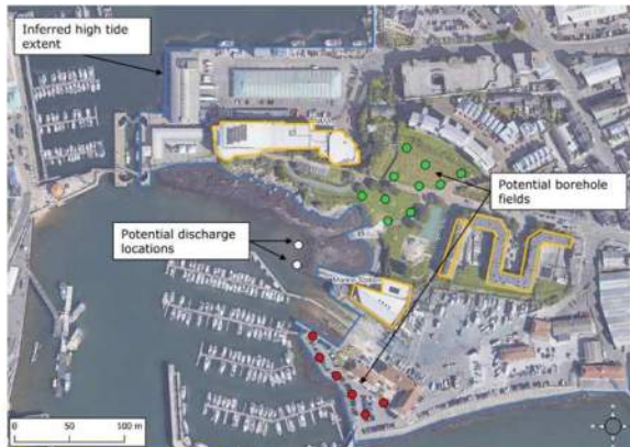
Figure 20: Open loop ground well opportunity in Sutton Harbour (Worley 2024)
